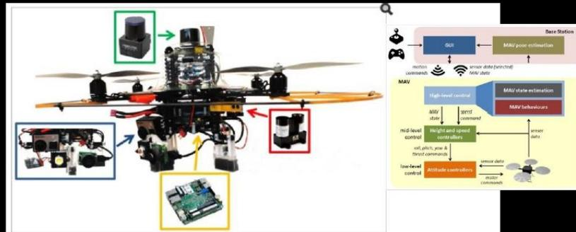
A realization of the INCASS aerial platform: (green) laser scanner; (red) height sensor; (yellow) embedded PC and (blue) camera set and illumination.
